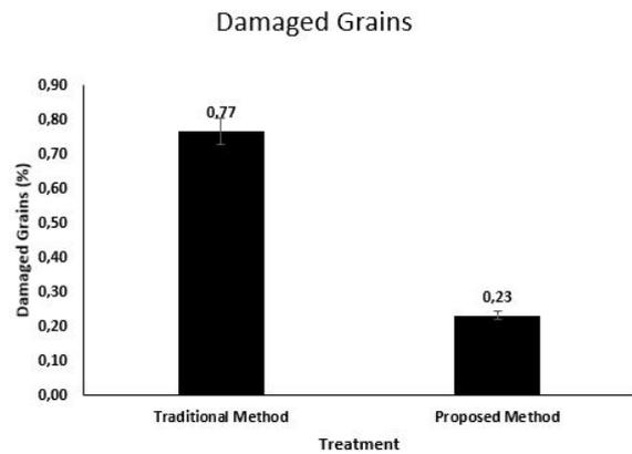
Figure 2. The percentages of damaged corn grains after treated with two different postharvest handling methods.
